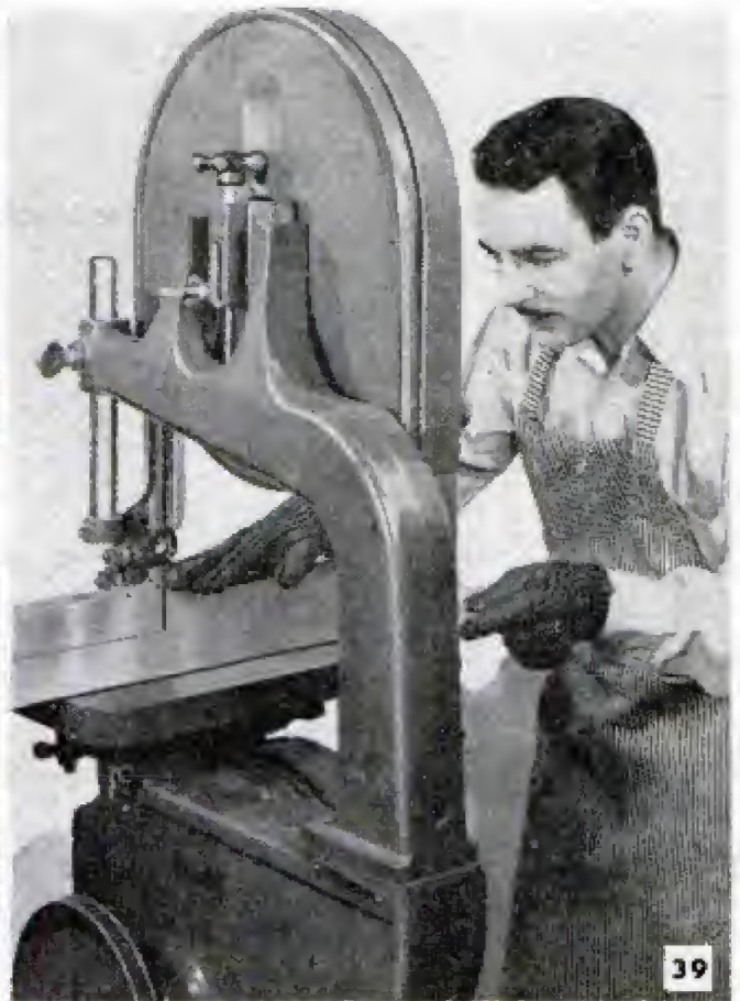
Bandsaw used as friction saw cuts fast and accurately on sheet metals of all kinds up to 1/8 in. thickness
